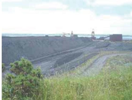
**Photo 1. Coal yard where the coal is stacked prior to being burnt**
